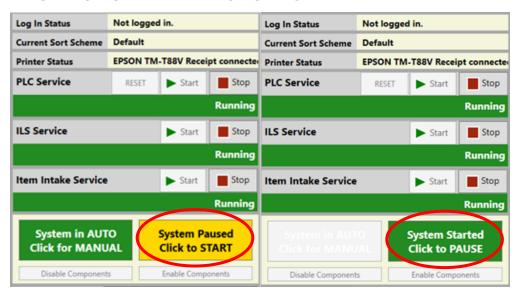
Once in Automatic mode, the system may be started by clicking the yellow button shown above. This button toggles the system between Running and Paused mode.
