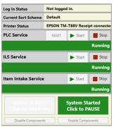
Pause/START - With the system in AUTO mode, place the machine in RUN bypressing the "System Paused, Press to START" button. Upon start up, the AMH conveyors will begin to move, indicating the system has been activated.
