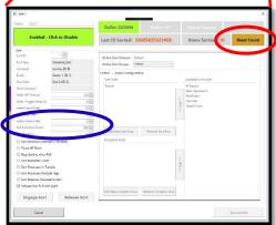
Periodically, as the system operates, the sorts will collect enough items to be designated as "Full". When this happens, an indicator light at the sort will light. Additionally, the corresponding sort button on the AMH screen will be colored blue. To reset the sort's Full Item Count and turn off the blue light, press the blue button at the sort zone or open the corresponding Sort Screen. Click on the orange 'Reset Count' button in the upper right corner. (Picture to the left – red circle)
