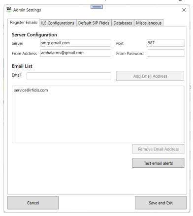
'Server Configuration' settings are at the top. Four fields are available to allow communication with an email server. Each is listed below along with information required.
