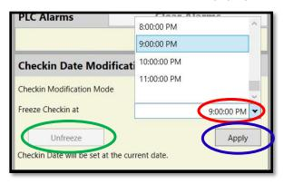
To deactivate Backdating or Freeze Checkin Date, simply click on the down arrow in the mode box, and select the 'None" option from the dropdown menu. Click the 'Apply' button to return the system to real-time item check-in. A confirmation will display in the lower left corner.
