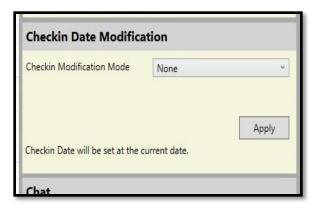
To enable Backdating or Freezing, click on the down arrow to display the dropdown menu. Select the desired check-in feature to present the viewable configuration choices. Below are instructions on how to activate as well as disable Backdating or Freeze Check-in Date. A key step in making sure the 'Check-in Date Modification' center records the desired date is to click the 'Apply' button. It ensures accurate returned dates.
