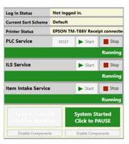
Pause/START - With the system in AUTO mode, place it into START by pressing the "System Paused, Click to START" button. Upon start up, the AMH conveyors
