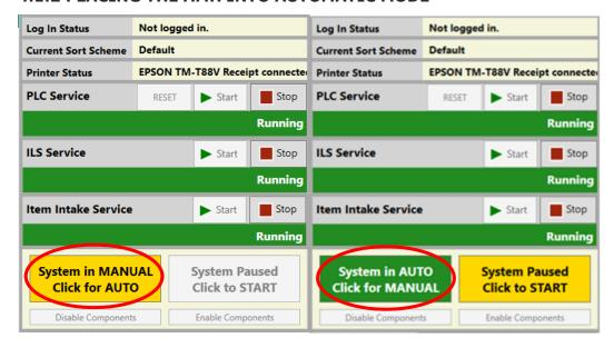
For the AMH system to run automatically, it must first be put into Automatic Mode. Upon start-up of the EZ Sort software the system will be in Manual Mode. Clicking the yellow button shown above will toggle the system between Manual and Automatic modes.
